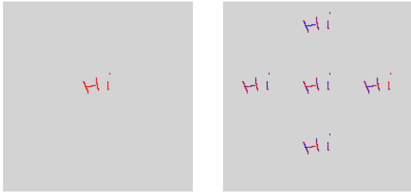
Figure 7: Starting from the initial configuration on the left, the modulo two rule is evolved for 64 steps using the four nearest neighbors. At a certain stage, five copies of the original image appear. The blue pixels indicate which sites were also alive one step before.
